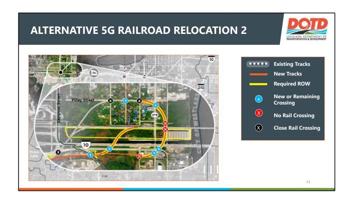
Railroad relocation #2 was identified as the option that would best serve all interests. As shown here, three existing crossings would be closed, and a total of six new or existing crossings would be improved with warning gates and flashers. The tracks south of Isle of Capri Boulevard, which are currently out-of-service, would be rehabilitated and put back into use for KCS.
