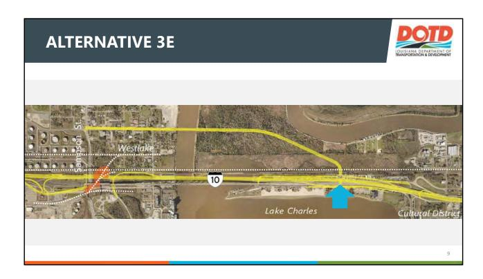
Alternative 3E differs from Alternative 3A only in that the interchange at North Lakeshore will be complete. That is, drivers can enter or exit the interstate from all directions by way of an extension of Sulphur Avenue. They may also use I-10 to cross the river entering or exiting at Sampson Street.
