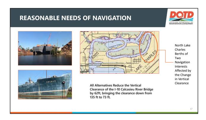
All bridges are considered navigation obstructions and are tolerated only as long as they serve the needs of land transportation and allow for the reasonable needs of navigation. Vertical clearance of the replacement I-10 bridge would be lowered from 135 feet to 73 feet. This clearance applies to all three alternatives.
