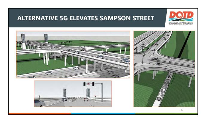
Random disruptions from freight trains that cross on the UP and KCS tracks at Sampson Street is a major traffic issue. Alternative 5G has the advantage of raising Sampson Street on structure and crossing over the railroads. It would also avoid the addition of a third movable bridge, which would cause random traffic disruptions.
