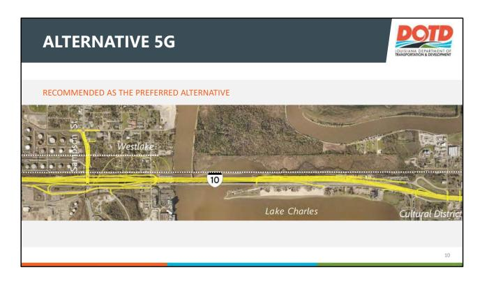
Alternative 5G was designed to provide a compact and complete interchange at Sampson Street. Sampson Street will be elevated to meet the interchange above I-10, eliminating the need for a Sulphur Avenue extension and moveable bridge to avoid the at-grade railroad crossings.
